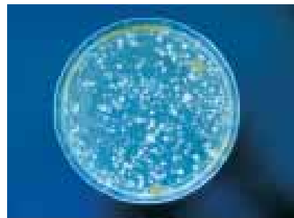
Dental treatment water biofilms - cleaned system in this image shows 1000,000 colony forming units per ml.
