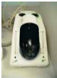
W&H Assistina is designed to clean and lubricate the W&H Handpieces prior to sterilization.
