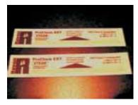
"Weekly" monitoring of the sterilizer's efficacy using Biological Equivalent monitoring devices or Sterilization Integrator (it measures whether the parameters of temperature and pressure over time) is necessary as this can be done in-house. The information should be recorded and maintained for a period of 3 years. The biological equivalents show color change when the sterilization parameters have
